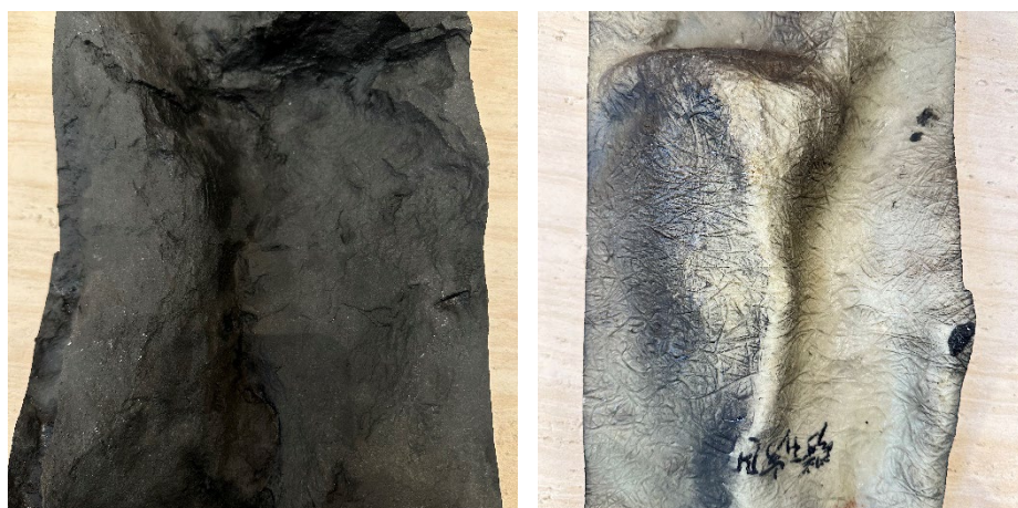
Figure 2: Representative specimen Textured Rock (Exposed face on left, reverse face on right)
